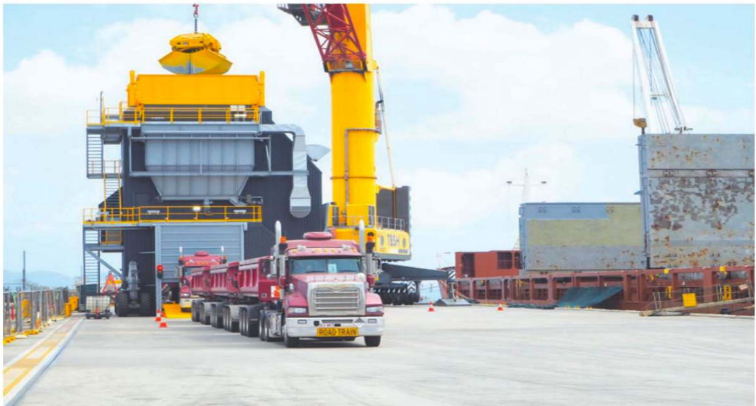
The hopper loading a triple road train for Sun Metals at Port of Townsville.
