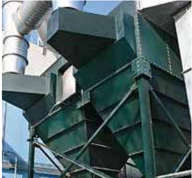
Cross flow is created through the filters. This eliminates upward “can” velocities associated with traditional hopper inlets.
