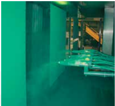
Farr Gold Series components are individually powder coated prior to assembly for superior corrosion resistance.
