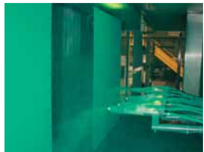
Individually Powder Coated Farr Gold Series components are individually powder coated prior to assembly for superior corrosion resistance.
