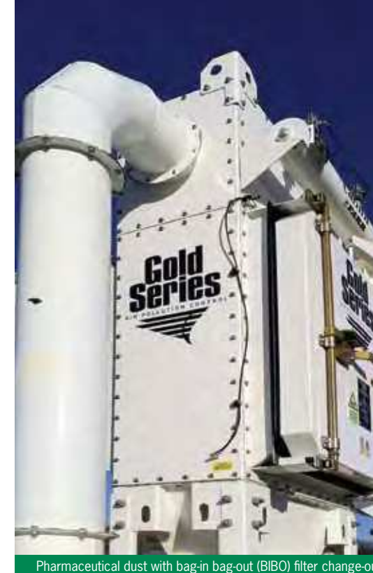
Pharmaceutical dust with bag-in bag-out (BIBO) filter change-out
