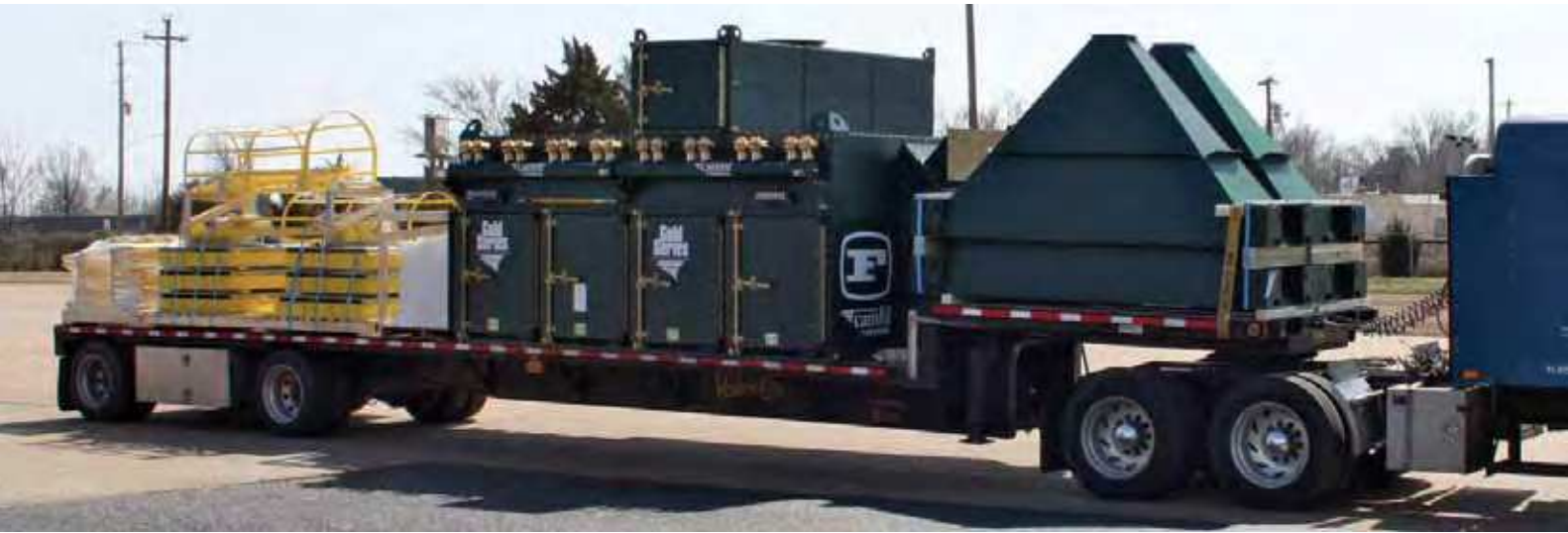
Custom Preassembled Skid Mounted Dust Extraction System
