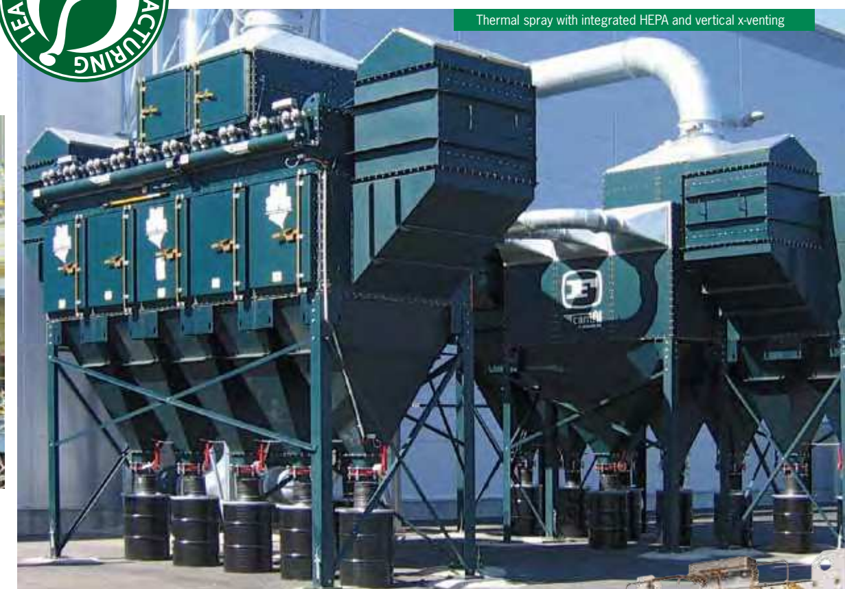
Thermal spray with integrated HEPA and vertical x-venting
