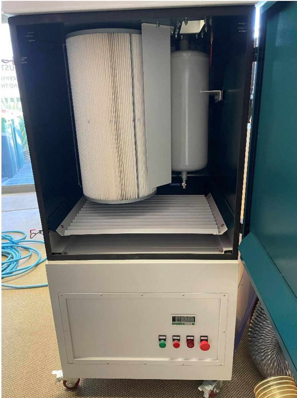
FILTER ELEMENT INSTALLED
